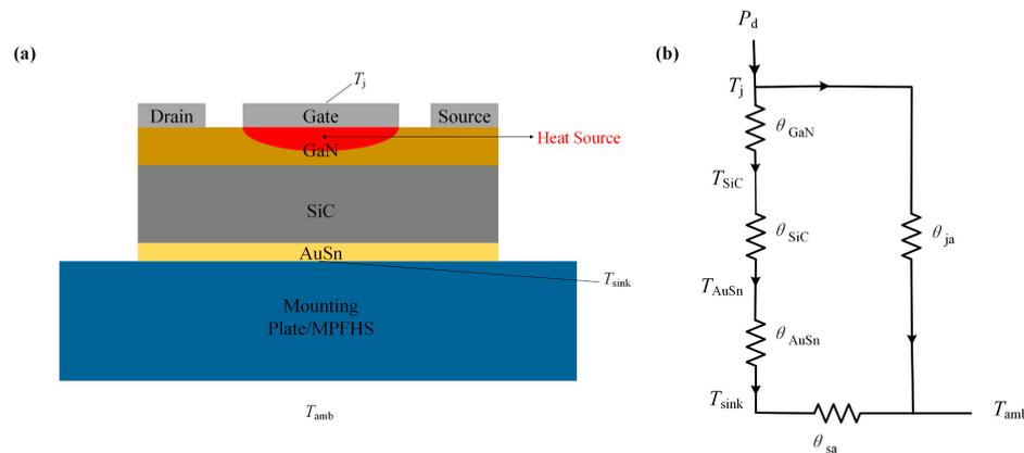
**Figure 5.** Thermal resistance model: (a) material system for the test module; (b) thermal resistance circuit for calculation and analysis.
