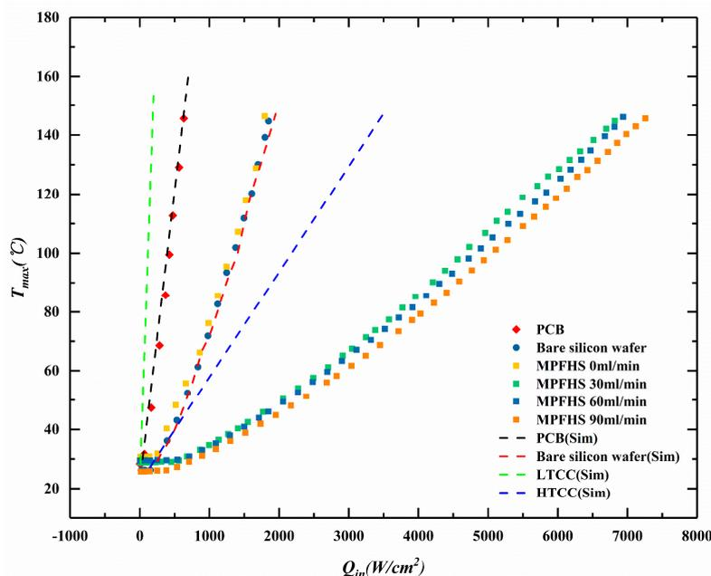
**Figure 6.** The maximum temperature of the GaN power amplifier mounted on three different plates (PCB, bare silicon wafer and MPFHS) as a function of dissipated power density probed by the IR camera system. During the experiments, the mass flow rates of the MPFHS were changed from 0 to 90 mL/min.
