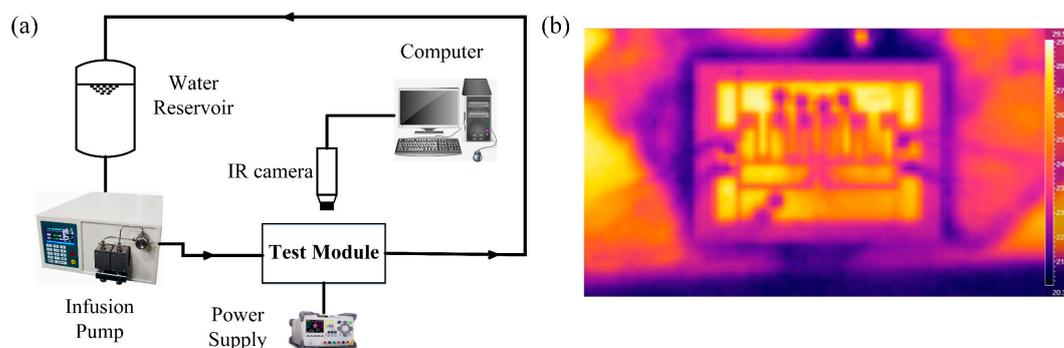
**Figure 3.** (a) Close-loop of the experimental test platform; (b) an IR camera was focused on the GaN power amplifier chips area (off working state).
