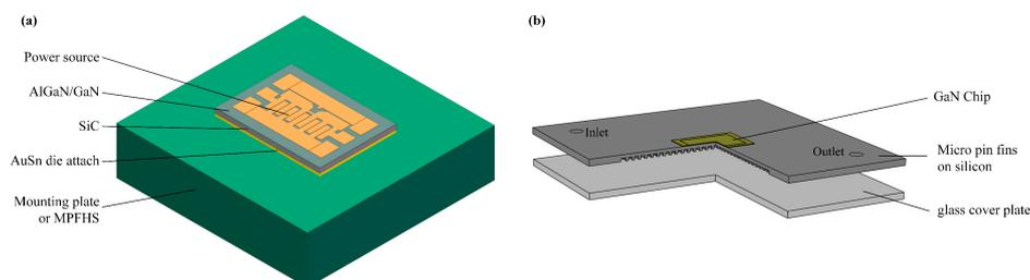
**Figure 1.** (a) Three-dimensional model of a GaN power amplifier mounted onto plates (not to scale), (b) Cross-sectional view of the GaN chip with integrated MPFHS (micro-pin fin heat sink) (not to scale).
