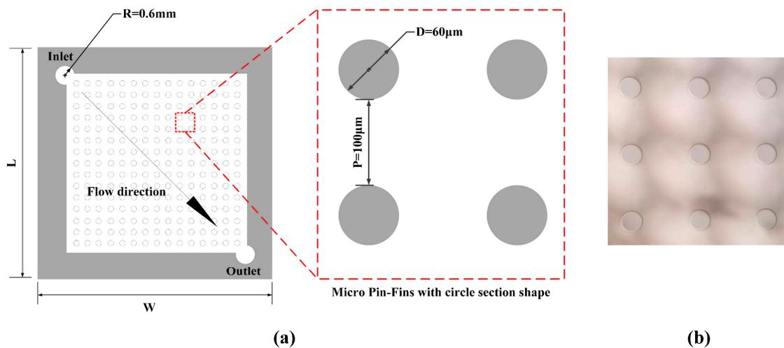
**Figure 2.** Si-based MPFHS: (a) schematic diagram of MPFHS; (b) microscopic image of an MPF (micro-pin fins).
