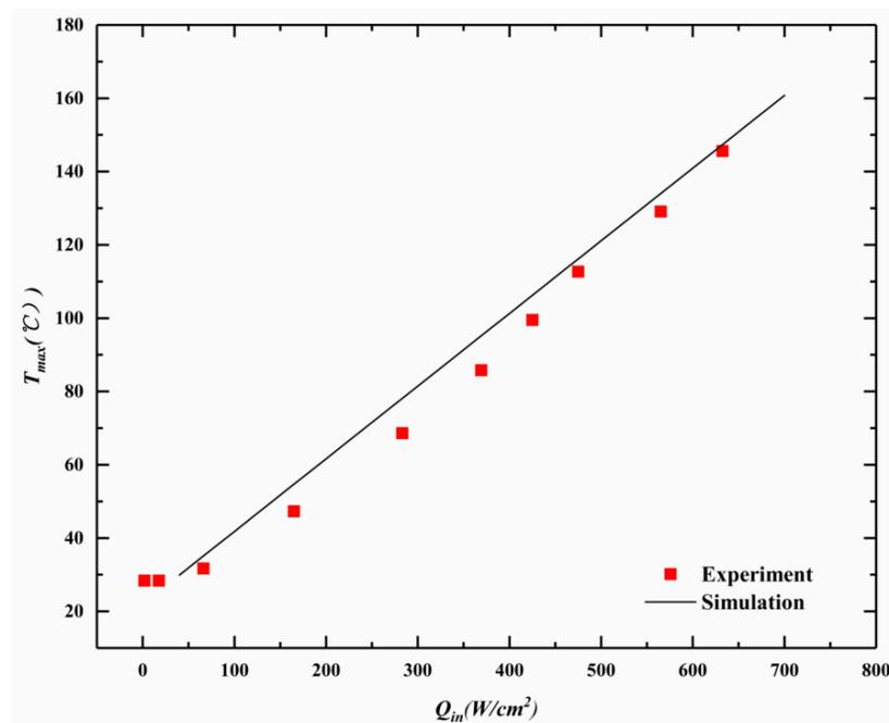
**Figure 4.** Maximum temperature of GaN chips (mounted on PCB) as a function of input power density obtained based on IR measurements and 3D FEM (finite element models) simulation results.
