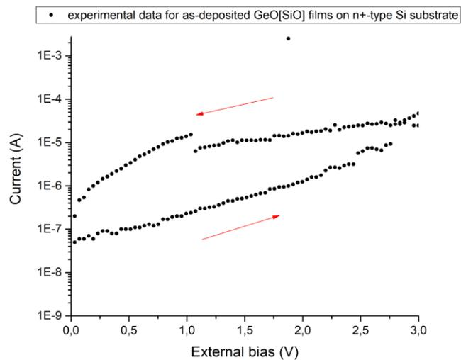
**Figure 4.** Exemplary experimental I–V characteristics of the as-deposited  $\text{GeO}[\text{SiO}_2]$ .
