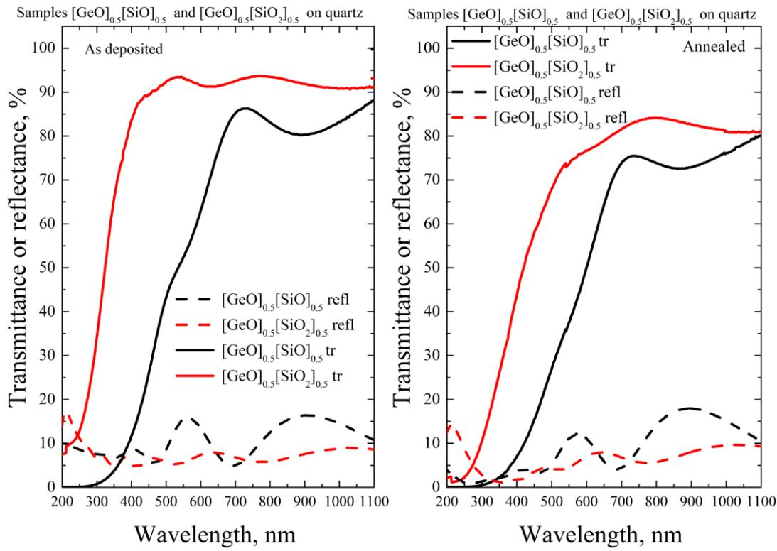
**Figure 3.** Transmittance and reflectance curves for  $\text{GeO}[\text{SiO}_2]$  and  $\text{GeO}[\text{SiO}]$  films on quartz substrates: (left) image–as-deposited films; (right) image–annealed films.
