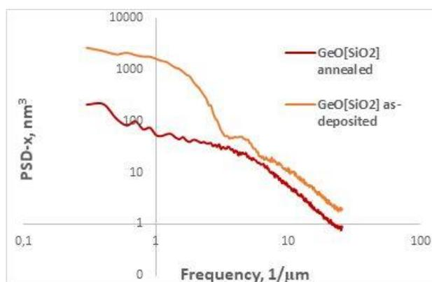
**Figure 2.** Power spectral density (PSD) of roughness measured for fast scan axis direction X shows small values of object sizes (X-axis,  $\text{nm}^3$ ) and amount of objects (Y-axis,  $\mu\text{m}^{-1}$ ) for the entire spectral range.
