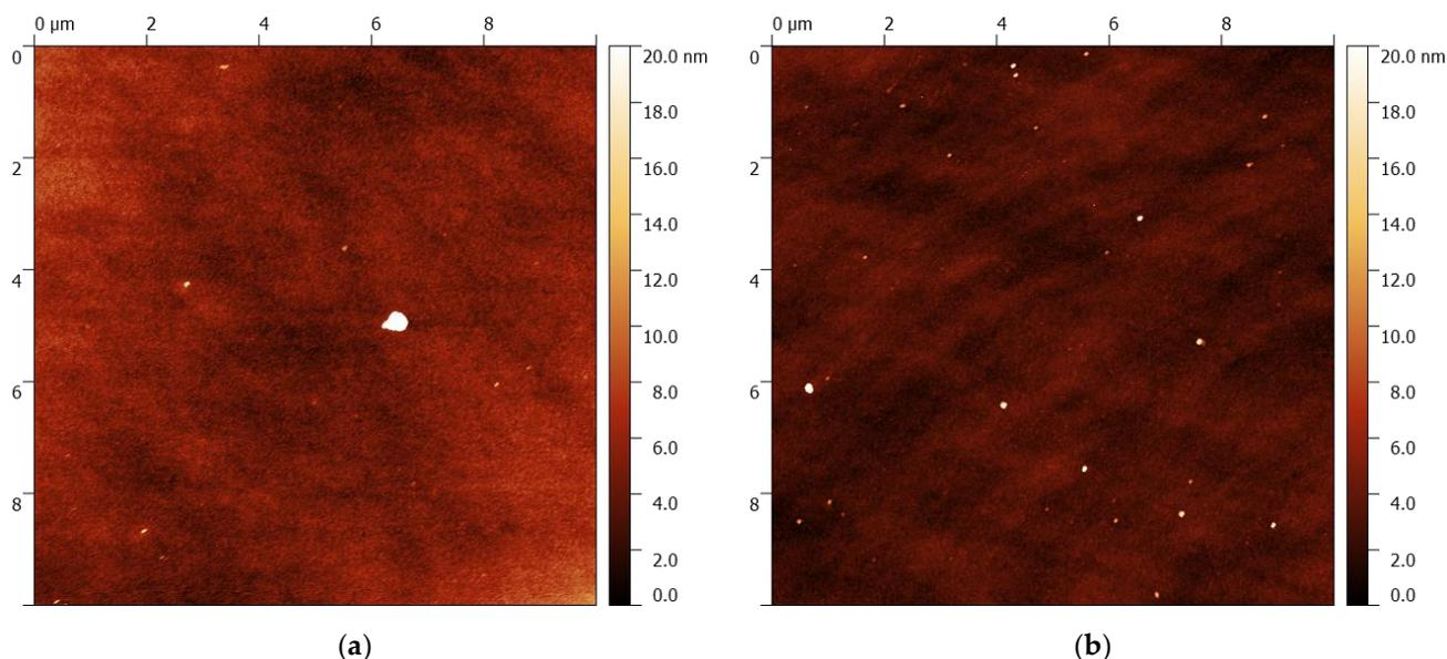
**Figure 1.** The 2D AFM topography images of the  $\text{GeO}[\text{SiO}_2]$  samples: (a) as-deposited; (b) annealed.
