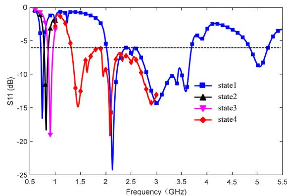
**Figure 5.** Simulated reflect coefficients of the proposed antenna for different diode states.
