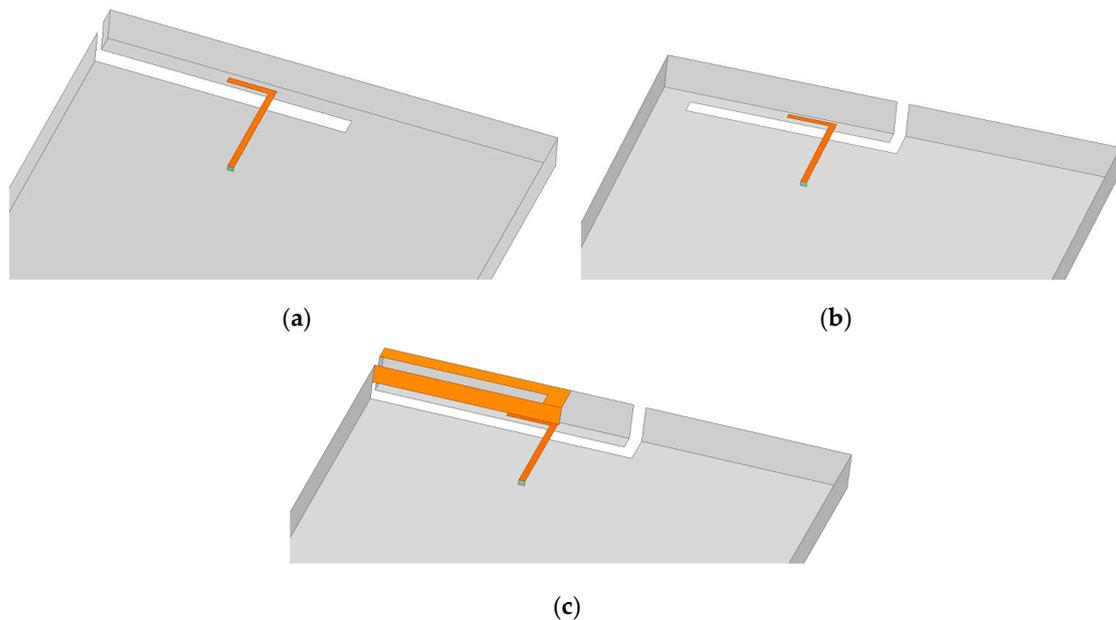
**Figure 3.** Evolution of the configuration. (a) Open-ended slot antenna with the open position at the long frame side; (b) open-ended slot antenna with the open position at the narrow frame side; (c) folded 3-D slot.
