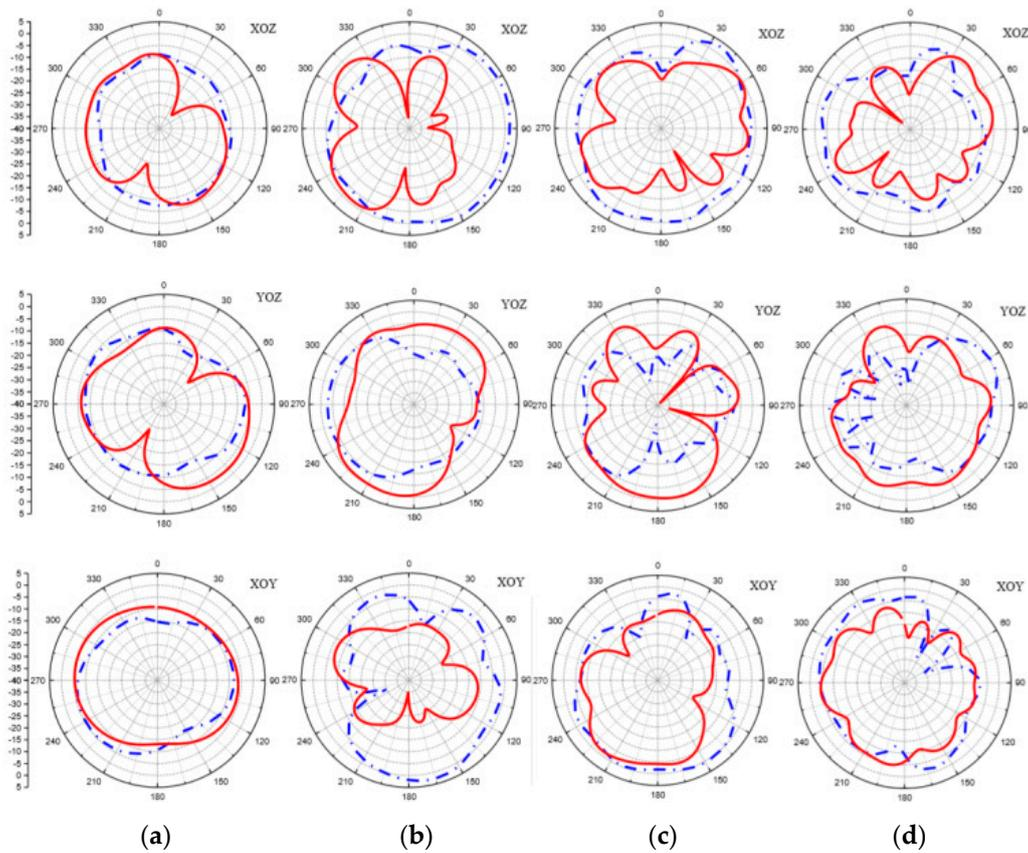
Figure 10. Measured 2-D radiation patterns of the proposed antenna at three principal planes (red solid line  $E_{\theta}$ , blue dashed line  $E_{\phi}$ , unit: dB): (a) 800 MHz; (b) 2100 MHz; (c) 3500 MHz; (d) 4900 MHz.
