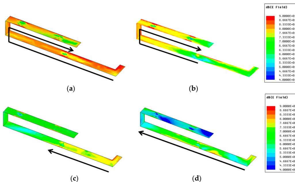
**Figure 4.** Electric field distribution of state 1 at different resonate modes: (a) 0.74 GHz ( $0.25\lambda$ ); (b) 2.1 GHz ( $0.5\lambda$ ); (c) 3.2 GHz ( $0.25\lambda$ ); (d) 5 GHz ( $0.75\lambda$ ).
