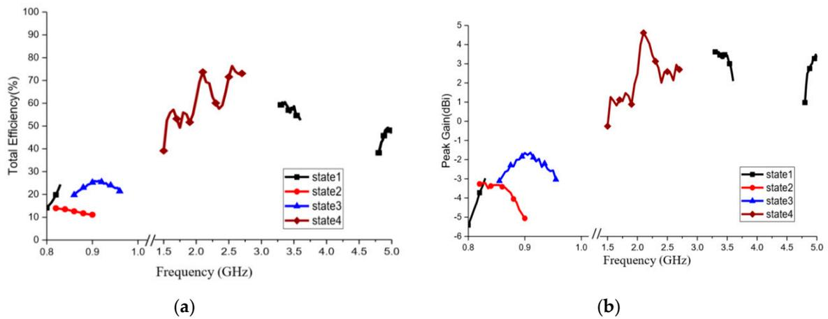
Figure 9. Measured efficiency (a) and gain (b).
