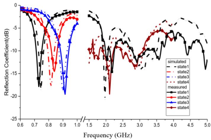
Figure 8. Measured reflection coefficient of different states.
