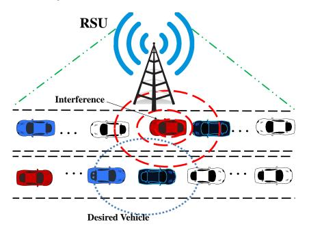
Figure 1. System model for V2V communications.
