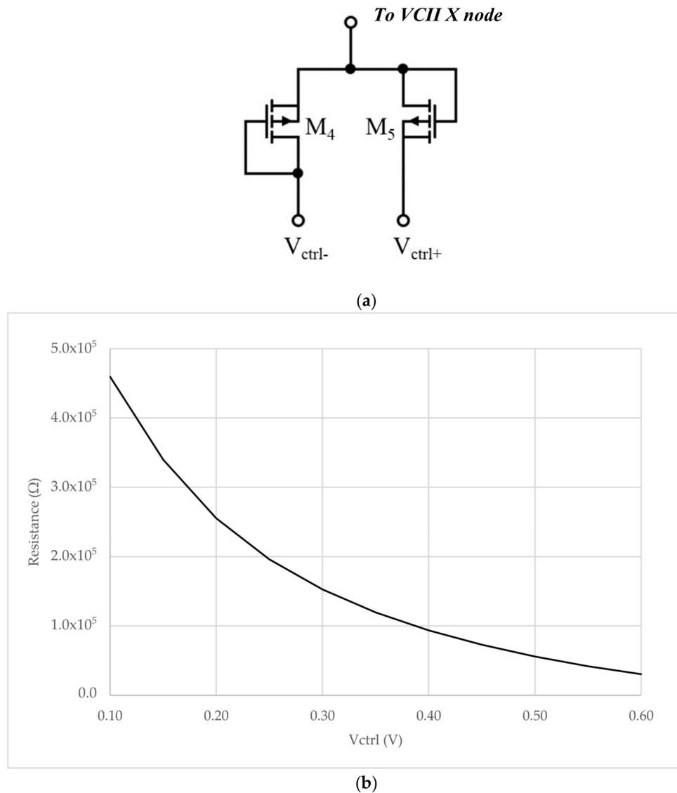
**Figure 5.** Implemented PMOS voltage-controlled shunt resistor  $R_g$  for neural amplifier gain tuning (a) circuit; (b) resistance vs. control voltage relationship.
