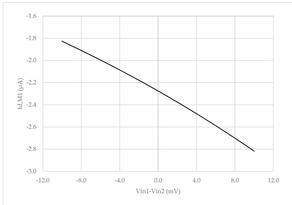
**Figure 7.** DFVF differential input voltage vs. output current relationship.
