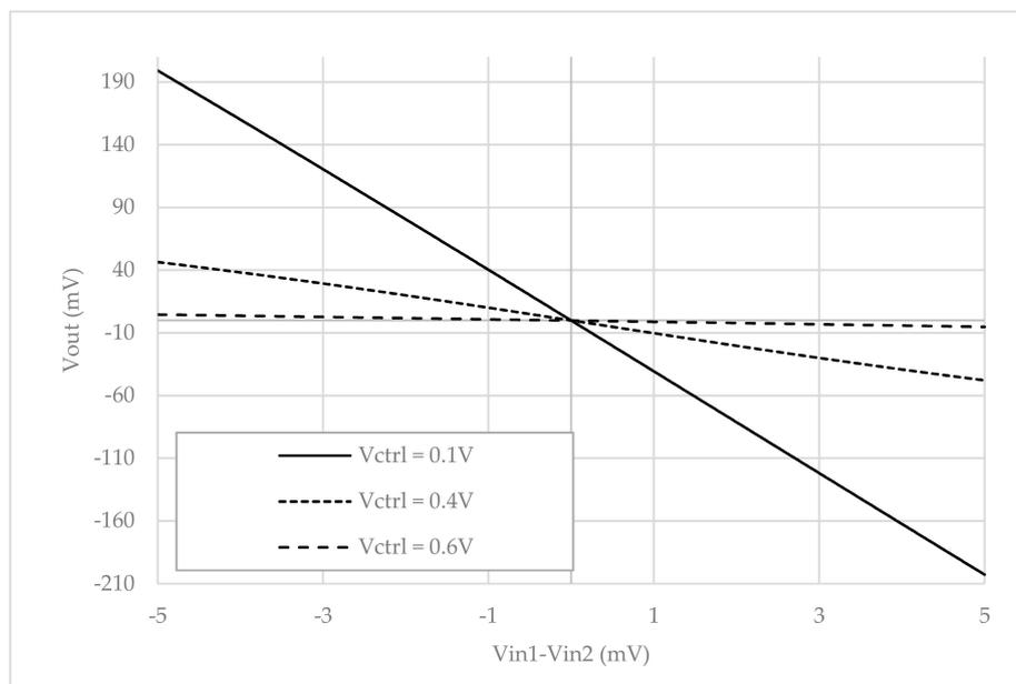
**Figure 9.** DC performances of the amplifier at various gain levels.
