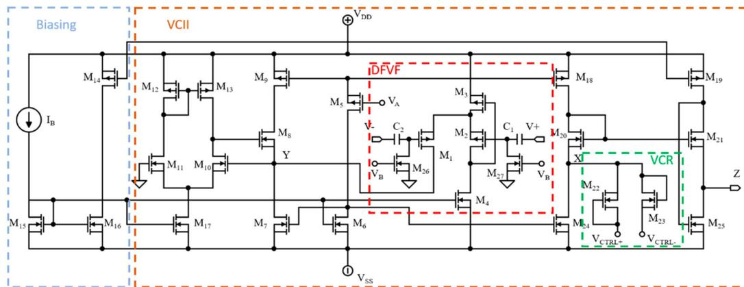
**Figure 6.** The complete transistor-level architecture of the proposed neural amplifier. The four main blocks have been highlighted: (1) Biasing current mirror (2) VCII complete block, (3) DFVF standalone block, (4) Voltage Controlled Resistor (VCR).
