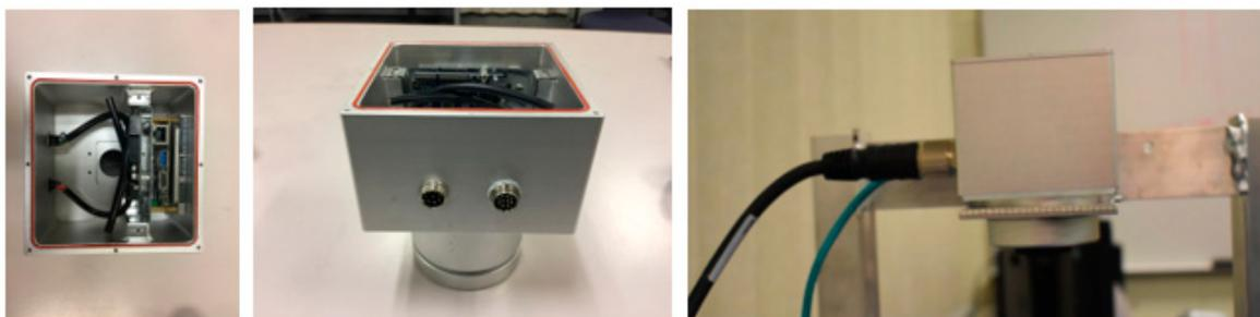
Figure 4. IP-64 enclosure of the smart camera.
