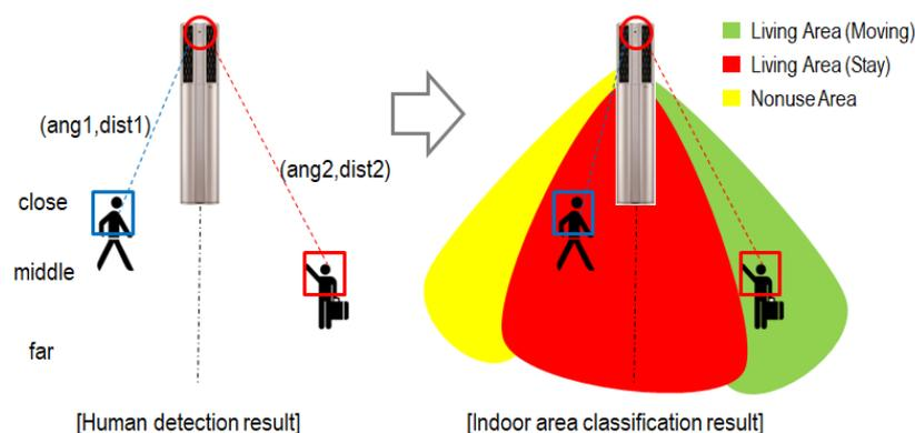
**Figure 1.** Examples of the Results of Human Body Detection and Indoor Space Area classification.
