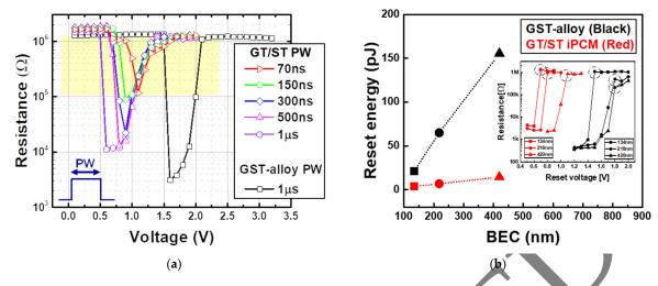
**Figure 2.** (a) A R–V graph of the GT/ST iPCM and Ge–Sb–Te (GST) alloy by the pulse width time, (b) a comparison graph of the reset energy by the bottom electrode contact (BEC) size (134, 218, 420 nm) between the GT/ST iPCM and GST alloy. The R–V graph in the figure shows the reset operation for each BEC size.
