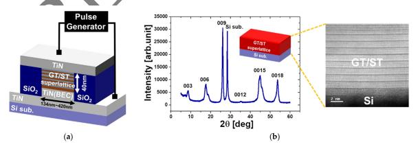
**Figure 1.** (a) Schematic of the fabricated GeTe/Sb<sub>2</sub>Te<sub>3</sub> (GT/ST) interfacial phase-change memory (iPCM) structure, (b) XRD diffraction pattern of a GT/ST SL (SL) structure and cross-sectional TEM image of the GT/ST superlattice on an Si (111) substrate.
