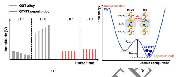
**Figure 3.** (a) Pulse scheme for long-term potentiation (LTP)/long-term depression (LTD) considering the mechanism of the GST alloy and GT/ST iPCM. (b) Schematic of the potential for Ge atoms of iPCM to diffuse in the reset and set states. The Ge atoms are shown in blue, Te atoms in yellow, and Sb atoms in orange.
