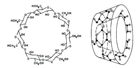
**Fig. 1.** The chemical structure of  $\beta$ -cyclodextrin molecule
