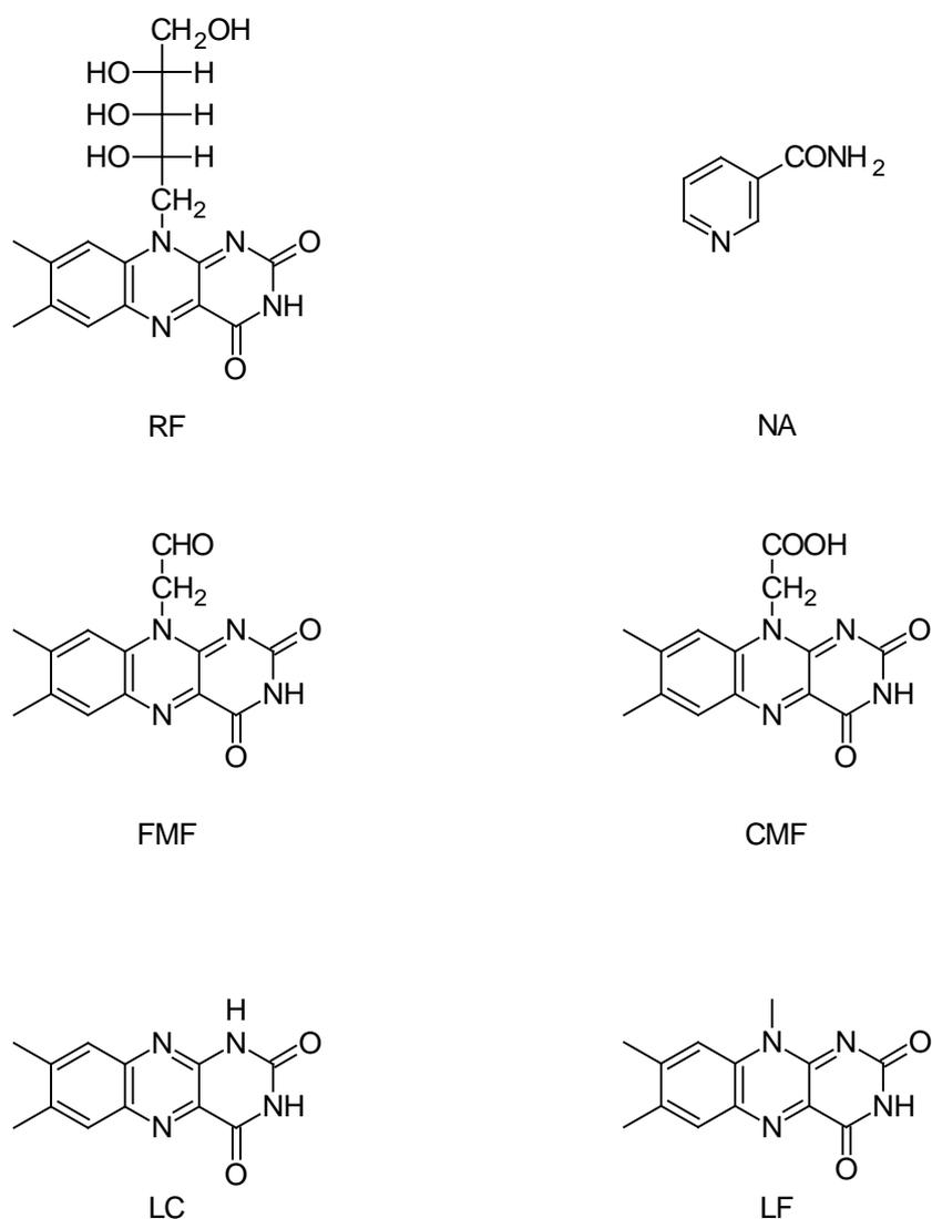
**Fig. 1.** Chemical structures of RF, its photoproducts (FMF, LC, LF, CMF) and NA.
