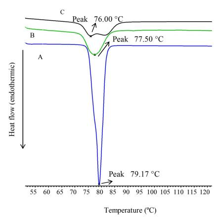
**Figure 5.** Differential scanning thermograms (DSC) thermograms of ibuprofen (**A**), alginate (**B**) and alginate–ispaghula (**C**) beads loaded with ibuprofen.
