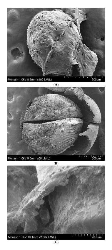
Figure 4. Surfaces of coated ibuprofen beads (A) were smooth. Cross-section of the bead clearly reveals formation of zein film (B) with a coating thickness of 8  $\mu$ m (C).
