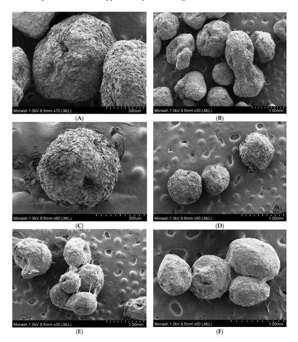
**Figure 3.** Field-Emission Scanning Electron Microscopy (FE–SEM) pictures of ibuprofen-loaded alginate (**A**,**B**) and alginate–ispaghula beads (**C**,**D**). Coating using zein is evidenced by bead adhesion and smooth surface of ibuprofen-loaded alginate (**E**) and alginate–ispaghula beads (**F**).
