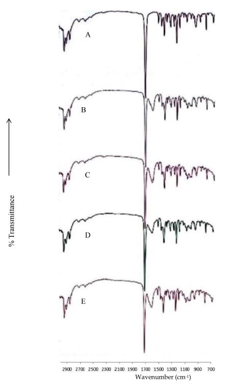
**Figure 2.** FT–IR spectrum of ibuprofen (**A**); alginate beads loaded with ibuprofen (**B**) and alginate–ispaghula beads loaded with ibuprofen (**C**); the spectrum of zein-coated alginate (**D**) and alginate–ispaghula (**E**) beads loaded with ibuprofen is also shown.
