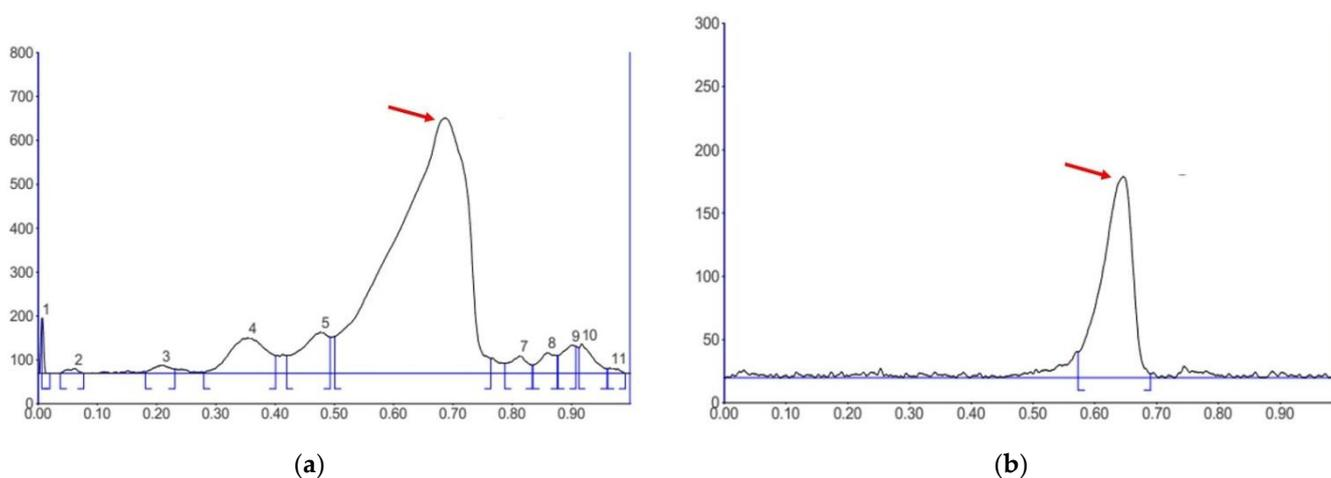
**Figure 2.** Quantification of brazilin in CSW ethanolic extract using TLC-densitometry analysis. Chromatograms of the CSW ethanolic extract (a) and brazilin standard (b) were obtained at a detection wavelength of 508 nm. A brazilin peak (red arrow) was observed with a maximum retention factor of 0.69. TLC-densitometry was conducted on silica gel F<sub>254</sub> as the stationary phase with chloroform:acetone:formic acid (4:2:0.5, v/v) as the mobile phase.
