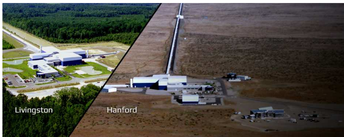
Figure 3. This is the picture of the Laser Interferometer Gravitational Wave Observatory, abbreviated as LIGO. There are two twin detectors in Livingston, Louisiana and Hanford, Washington separated by 3000 km. The arm length is 4 km. (Image credit: LIGO)
