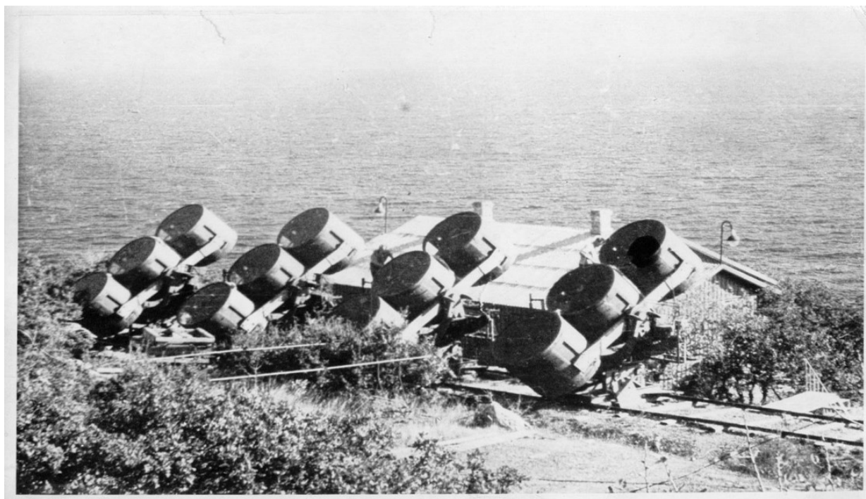
Figure 3. The telescope of A. Chudakov and colleagues in Crimea near the Black Sea shore.
