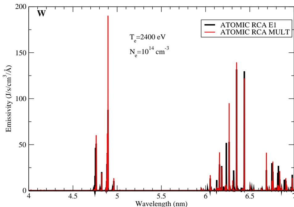
**Figure 2.** Emission spectrum of tungsten at a temperature of 2400 eV and an electron density of  $10^{14} \text{ cm}^{-3}$ . ATOMIC RCA E1 calculations (black curve that includes only electric dipole transitions) are compared with ATOMIC RCA MULT calculations (red curve that includes radiative transitions up to and including M3).
