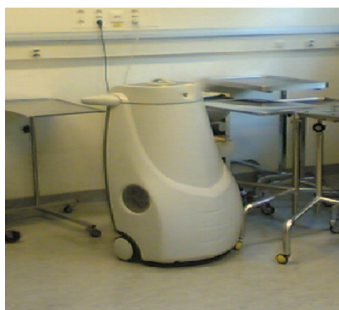
Figure 3. Decontamination of rooms and equipment with a hydrogen peroxide aerosol, using a pre-programmed robot (Reproduced with permission from: Andersen et al. [18] [Journal of Hospital Infection]).
