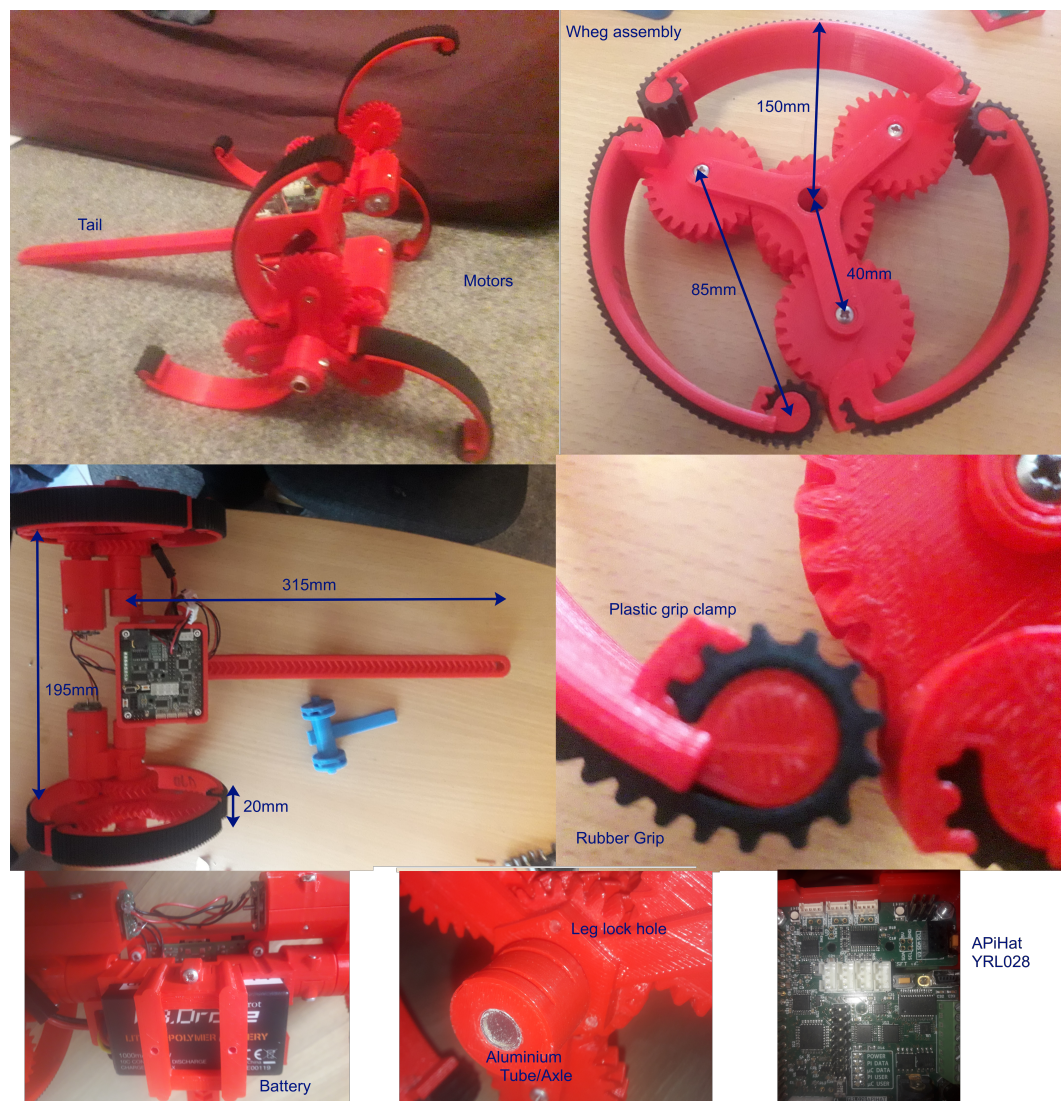
Figure 1. Top left: Cyclindabot with legs fully deployed and end of aluminium axle shaft showing. Top right: Three limbed Wheg design detached from the robot. Middle left: View of Cyclindabot from above with blue scale model from design process. The PCB of controller hat and 20D motors also visible. Middle right: Close up on herringbone gear and rubber grip attachment. Bottom left: Underside of robot and battery. Bottom middle: End of aluminium tube that acts as the axle for the Wheg assembly and the holes for locking the leg angles. Bottom right: Close up on the APiHat PCB.
