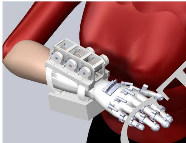
Figure 6. 3D CAD model of the hand exoskeleton.
