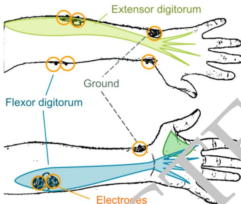
**Figure 8.** The sensor location of the EMG electrodes on the human forearm, including the anterior surface and posterior surface.
