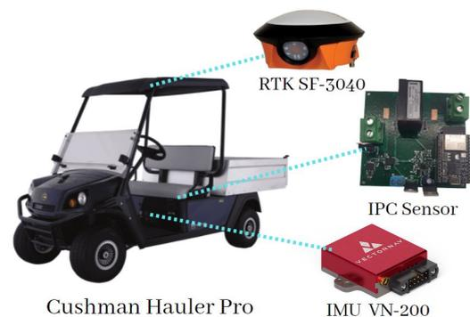
**Figure 8.** Electric vehicle used for field testing, equipped with an RTK system, an IMU, and an IPC (voltage and current) sensor connected to the batteries.
