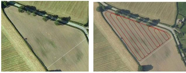
The field used is located at 52.42° N, 2.58° W, and the dimensions were sampled from Google Earth and scaled down by 1:14 to be relative to the test platform. The route was planned using a working width of 0.714 m (approximately, in full scale, 10 m) and driving parallel to the longest edge of the field.
