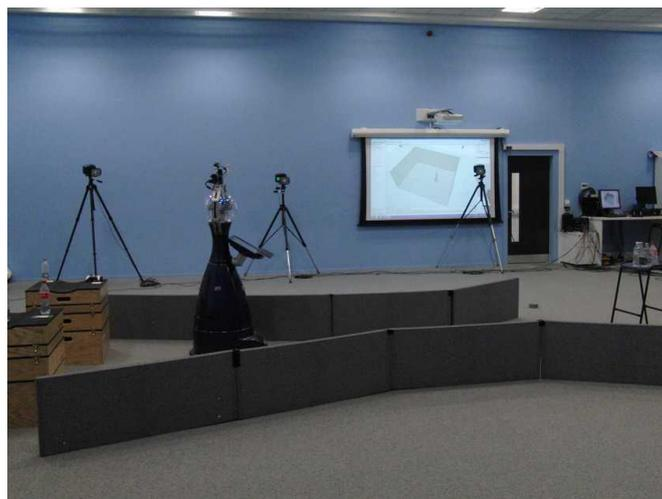
**Figure 9.** The “Lincoln experiment” set-up showing the robot, the motion capture cameras, the artificial corridor, and the “tables” and “kitchen counter”. The shown set-up elicits close encounters between human and robot in a confined shared space to investigate their interaction.
