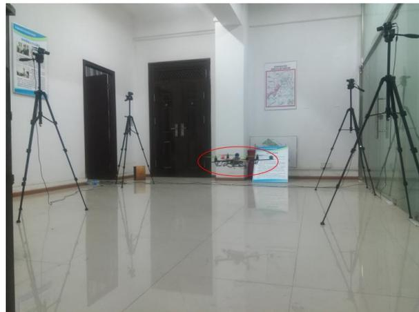
Figure 7. The multi-camera measurement system and the testing MAV.
