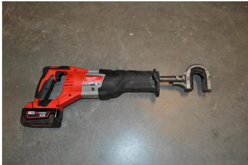
**Figure 8.** Hand held shaker used for cherry branch shaking.
