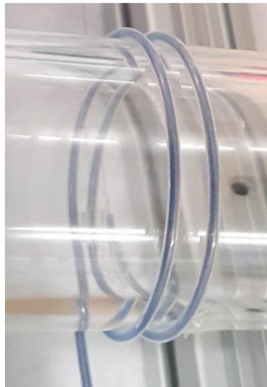
**Figure 5.** Lubricant experiment. Example of lubricated tube-guided SMA wire actuator. In this case, the guiding tube has been lubricated with fine graphite powder.
