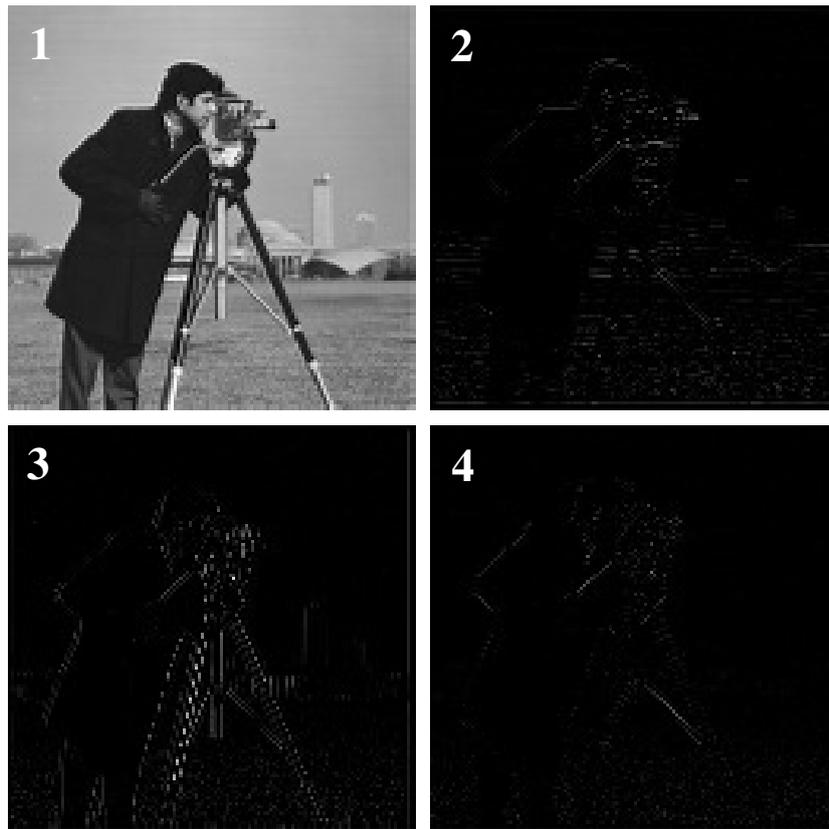
**Figure 7.** The wavelet decomposition of the reference image approximation-horizontal, vertical, and diagonal coefficients [38] (© 2018 IEEE).
