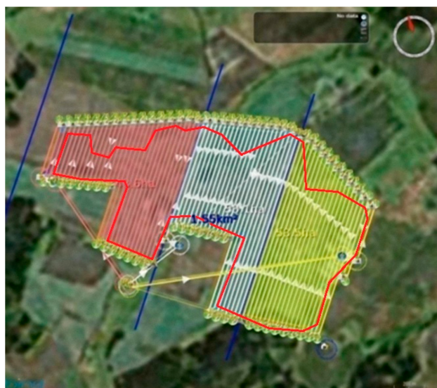
Figure 4. Flight plan for UAV mapping of the built-up area of the village of Tymákov. The entire area was divided into three blocks (marked with pink, white and yellow) to maximise UAV endurance. The red line indicates the border of the area to be mapped (155 ha).
