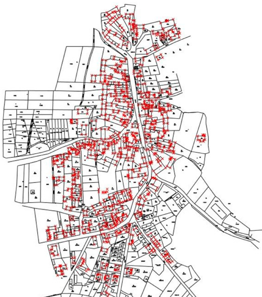
Figure 12. Identical points (red crosses) measured in the point clouds derived by image matching and geodetic survey (GNSS-RTK and total station) in the Soběšice u Sušice test area.
