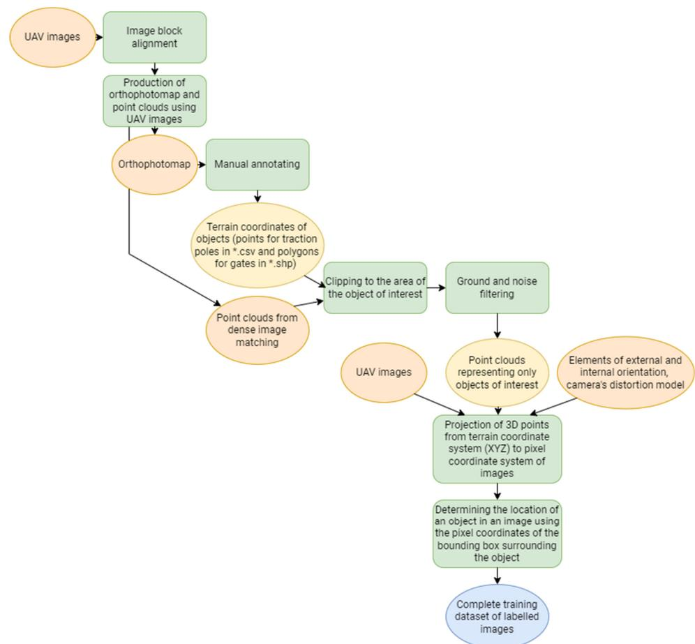
Figure 9. Workflow to semi-automate the process of preparing training datasets for object detection.
