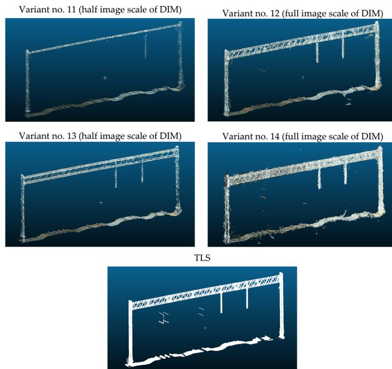
**Figure 1.** Point cloud fragments clipped to the gate object for all analyzed variants.
