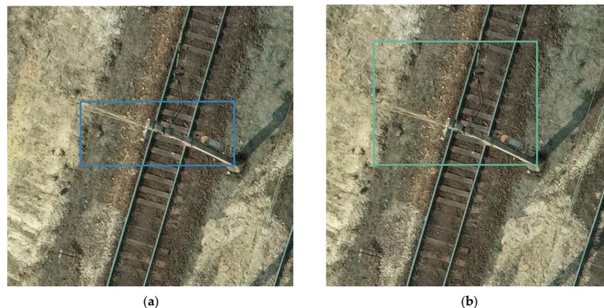
**Figure 16.** An example of a training dataset for traction poles with IoU = 0.48; (a) the bounding box generated from DIM point clouds; (b) ground-truth bounding box from TLS point cloud.
