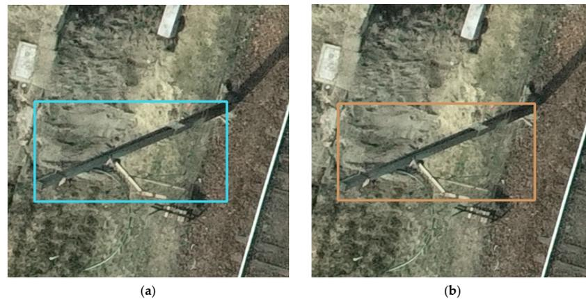
**Figure 15.** An example of a training dataset for traction poles with IoU = 0.94; (a) the bounding box generated from DIM point clouds; (b) ground-truth bounding box from TLS point cloud.
