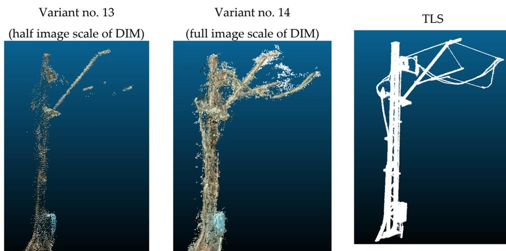
**Figure 2.** Point cloud fragments clipped to the traction pole object for all analyzed variants.
