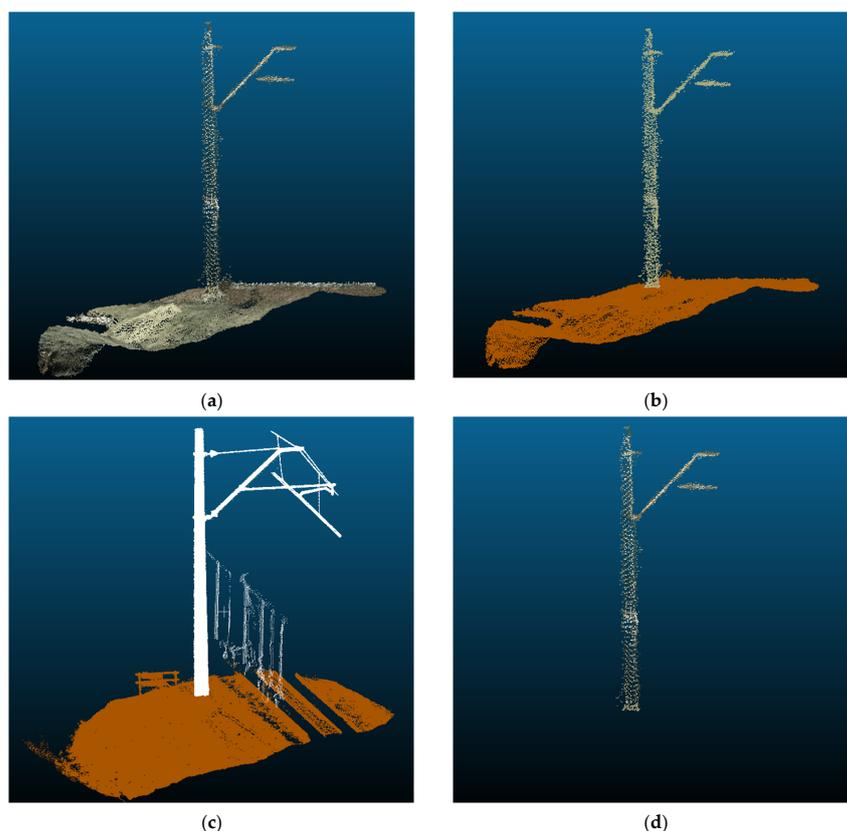
**Figure 5.** Cloth Simulation Filter (CSF) ground filtration examples: (a) an example of the source cloud, (b) the same object after ground filtration colored by classes—ground and non-ground, (c) an example of ground filtration for a point cloud with TLS, (d) the final segment of the point cloud passed to the next stage of the algorithm.
