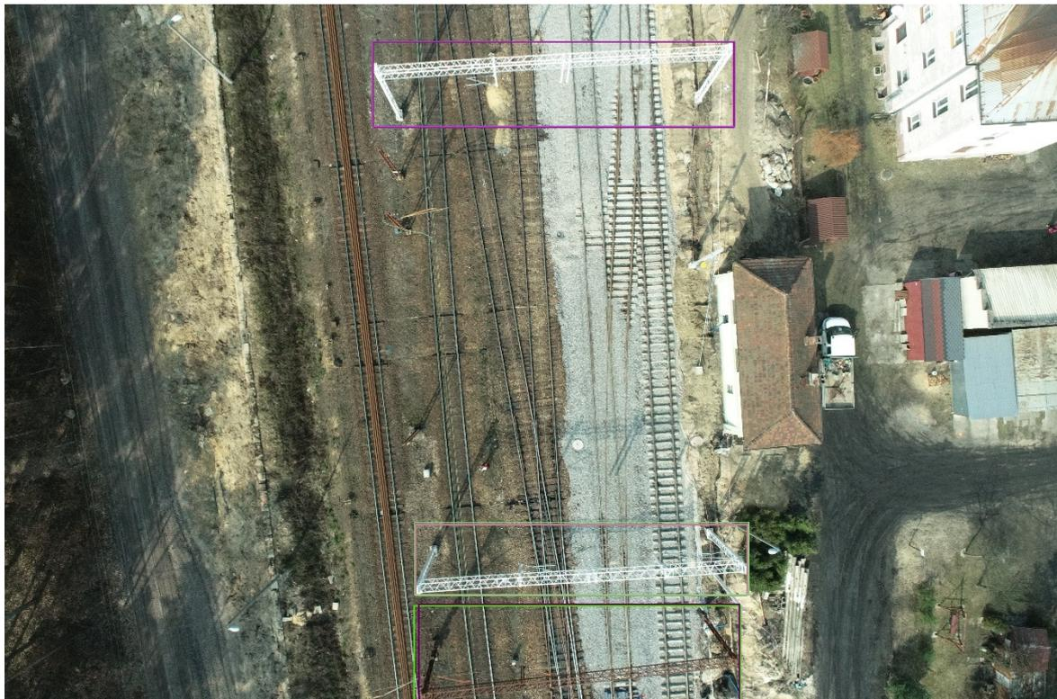
**Figure 17.** An example of comparing bounding boxes for gates obtained using automatic generation from ground-truth for the entire image. From the top, IoU values: 0.9935, 0.9698, 0.9629.
