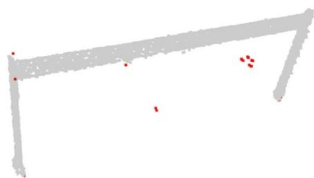
**Figure 6.** An example of noise filtering for a gate, where the red points are noise and the gray points are the object.
