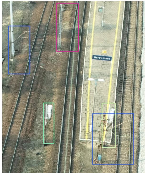
Figure 8. The final result is an example of training dataset for traction pole detection.
