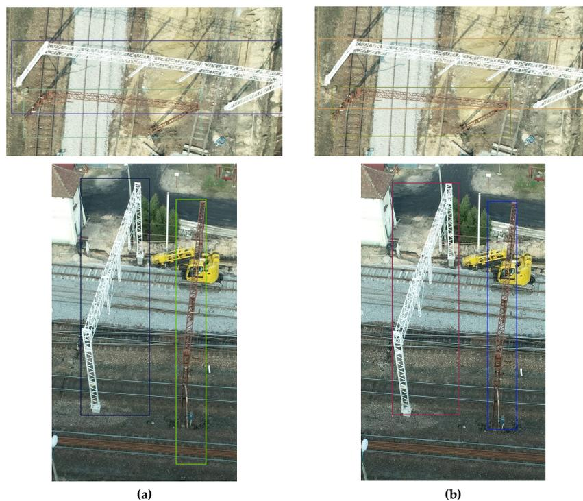
**Figure 11.** Example results for gates: (a) bounding boxes obtained from point cloud from DIM, (b) ground-truth bounding boxes obtained from point cloud from TLS.
