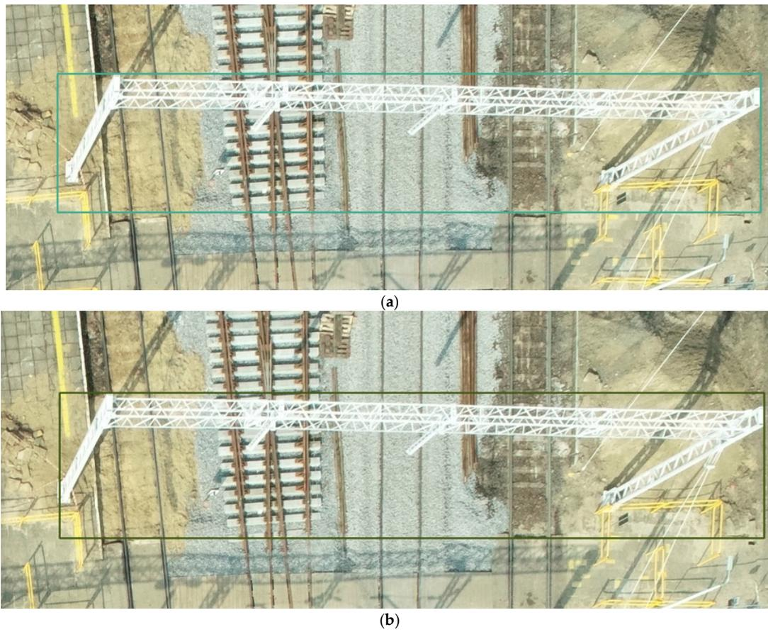
**Figure 13.** An example of a training dataset for gates with  $\text{IoU} = 0.90$ ; (a) the bounding box generated from DIM point clouds; (b) ground-truth bounding box from TLS point cloud.
