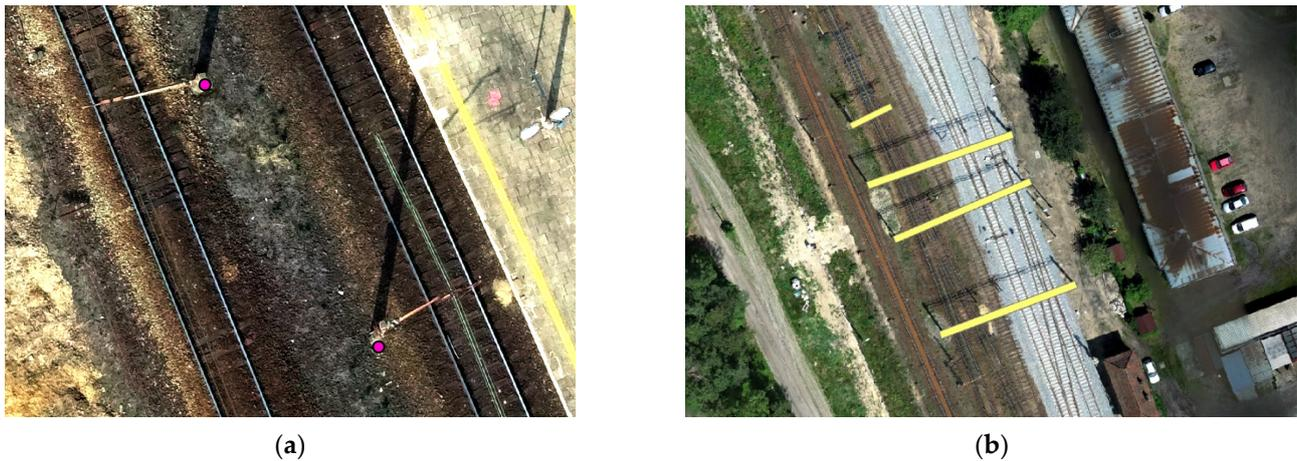
**Figure 3.** Examples of annotation data for (a) traction poles annotated as points and (b) gates labelled as polygons based on orthophotomap from UAV images.
