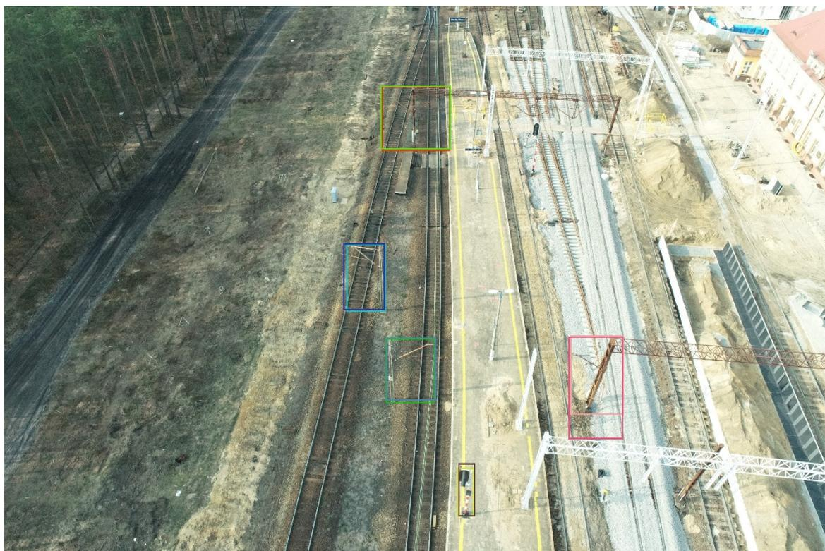
**Figure 18.** An example of comparing bounding boxes for traction poles obtained using automatic generation from ground-truth for the entire image. From the top, IoU values: 0.9748, 0.9116, 0.9675, 0.7411, 0.8496.
