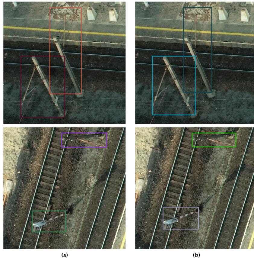
**Figure 10.** Example results for traction poles: (a) bounding boxes obtained from point cloud from DIM, (b) ground-truth bounding boxes obtained from point cloud from TLS.
