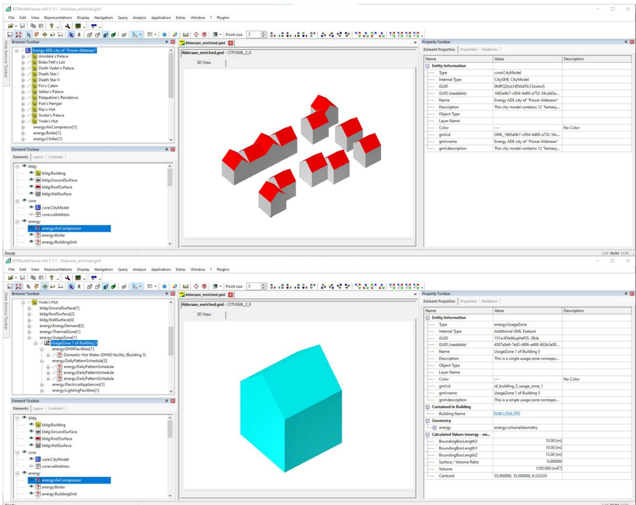
**Figure 30.** Visualisation of the test dataset in the FZK ModelViewer. Upper picture: the CityModel with its LOD2 buildings and properties. Lower picture: the *UsageZone* of Building “Yoda’s Hut” with its properties and own geometry.
