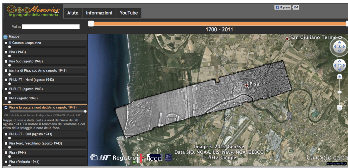
Figure 9. The GeoMemories application. Note the Google Earth navigation tools on the right, the slider to select a time frame on top, and the historical map selector on the left. One historical map is chosen, which is composed of several photos taken by RAF during a flight in August 1943 over the city of Pisa in Italy. (©MiBAC-ICCD, Aerofototeca Nazionale, fondo RAF. ©2010 Google).
