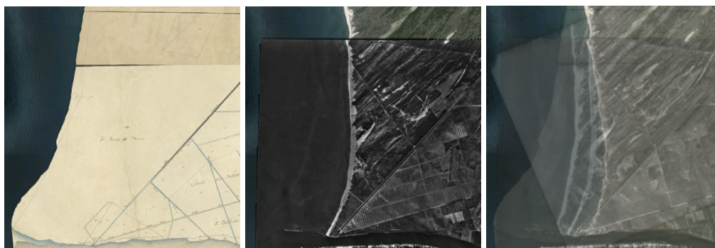
Figure 13. Snapshots of the mouth of the river Arno, near Pisa. Left: A cadastral map from 1765. Middle: Aerial photo from 1962. Right: An overlay of the cadastral map, the historical photos from 1943 and 1962 and the Google Earth modern satellite photo. The user can visually perceive in a single image the changes in the coastal line throughout two and a half centuries (©MiBAC-ICCD, Aerofototeca Nazionale, fondo RAF. ©2010 Google).
