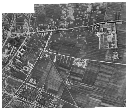
Figure 8. Two photos are stitched together using the transformation computed from the corresponding points (green crosses in Figure 1) in the overlapping area. (©MiBAC-ICCD, Aerofototeca Nazionale, fondo RAF).
