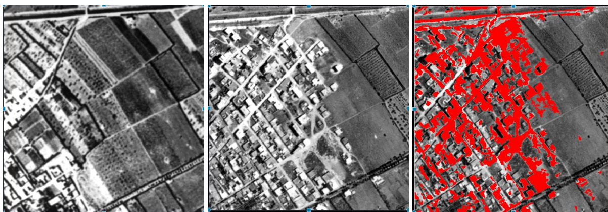
Figure 2. An example of the result obtained by running an automatic change detection algorithm on the first two images, representing the outskirts of Pisa in 1954 and 1968. Urban expansion over 14 years is highlighted in red in the picture on the far right (©MiBAC-ICCD, Aerofototeca Nazionale).
