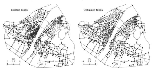
Figure 3. Distribution of existing and optimized bus stops.
