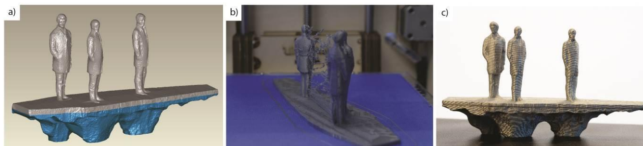
Figure 9. (a) Both parts of the completed mesh model, with the lower part shown in blue, (b) the top part of the model in the ELRP machine; (c) and the completed physical model.
