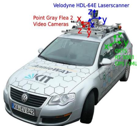
**Figure 6.** The sensor configuration on the platform (courtesy of [25,26]).
