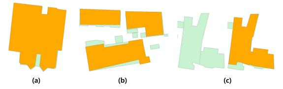
**Figure 4.** Examples of labeled buildings: (**a**) 0-eliminated; (**b**) 1-retained; (**c**) 2-aggregated (green = 1:1000 scale; orange = 1:25,000 scale).
