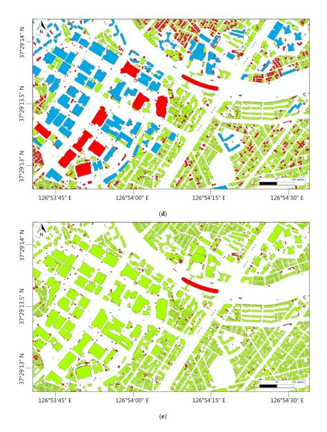
**Figure 7.** Visualized results of each algorithm: (**a**) original class, (**b**) DT, (**c**) *k*-NN, (**d**) NB, and (**e**) SVM. Blue = eliminated (0); green = retained (1); and red = aggregated (2).
