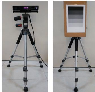
**Figure 5.** Setup of the method: Kinect v2 (left); stripe plane pattern (right).
