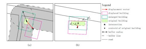
Figure 15. Determination of the building displacement vector for: (a) a C-type building; (b) an E-type building.
