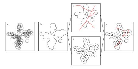
**Figure 11.** Extraction of selection units: (**a**) building buffering; (**b**) merging of buffered polygons; (**c**) conducting an overlap with roads; (**d**) conducting an overlap with buildings; (**e**) assigning buildings and roads to form selection units.
