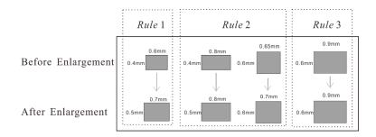
Figure 12. Three rules for enlargement of individual buildings at scales of 1:25,000 and 1:50,000.
