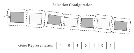
**Figure 6.** Encoding for a group of aligned buildings. *r*′ is half the minimum distance threshold for detecting conflicts.
