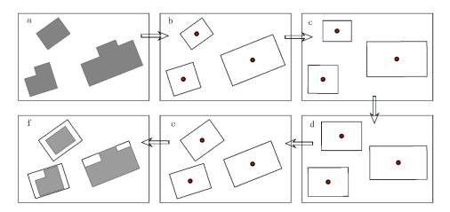
**Figure 13.** Building enlargement process: (**a**) original buildings; (**b**) SMBRs; (**c**) first rotation; (**d**) simple geometric transformation; (**e**) second rotation; (**f**) buildings after enlargement compared to their initial states.
