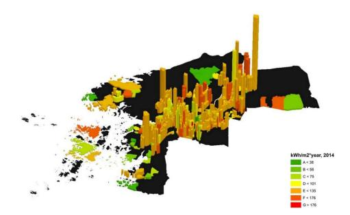
**Figure 6.** 3D visualization of energy performance and total energy use in aggregated–base areas. The color of the bar represents the average energy performance using the scale from the EPC [ $kWh/m^2$ ] while the height represents the total energy use of buildings in the different statistical areas [GWh].
