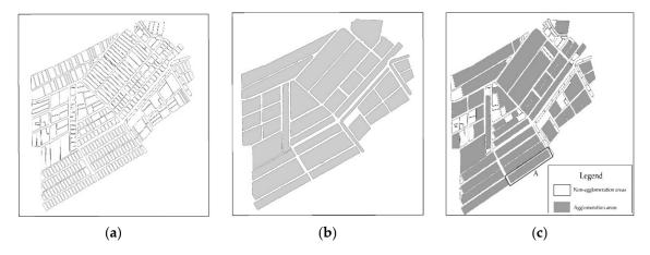
**Figure 18.** Identification and processing of the agglomeration areas: (a) Original pond data; (b) candidate agglomeration area and (c) first-stage agglomeration areas.
