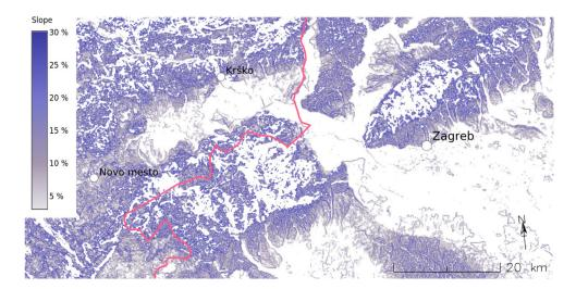
**Figure 9.** Areas filtered by slope criteria. Flat and too steep areas, as well as areas with very low and very high variation of the slope, are excluded (white).
