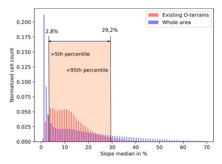
**Figure 7.** Histograms of the slope median determined for the spatial neighborhood, defined as a circular area with a diameter of 15 pixels, with cut off values determined from existing O-terrains then applied to the whole area.
