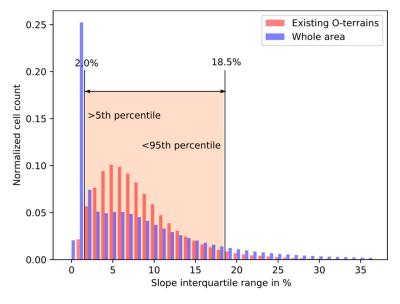
**Figure 8.** Histograms of the slope interquartile range determined for the spatial neighborhood, defined as a circular area with a diameter of 15 pixels, with cut off values determined from existing O-terrains then applied to the whole area.
