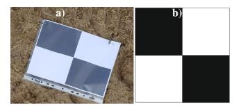
**Figure 7.** (**a**) Ground Control Point marked in the field with a white and black chessboard; (**b**) Project of the ground control point.
