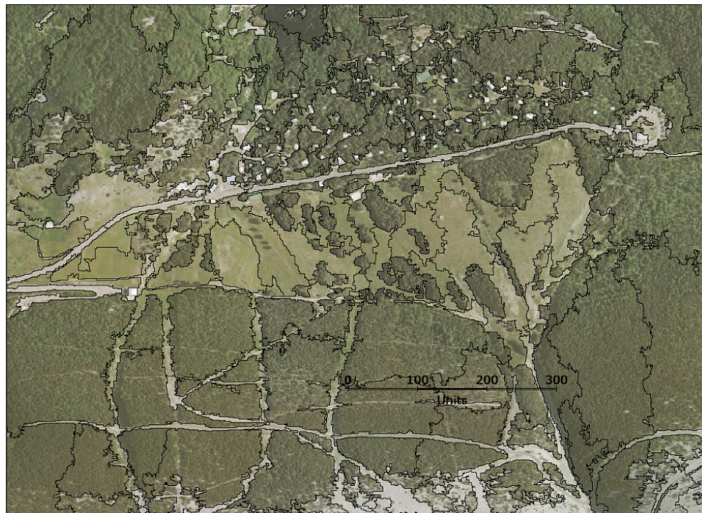
Figure 4. Segmentation obtained using Baatz and Schäpe algorithm with scale 70 (BS-70).
