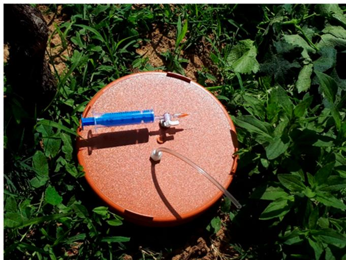
**Figure 9.** Closed-system static chamber for gas sampling with injection syringe and needle (photo by L. Horváth).
