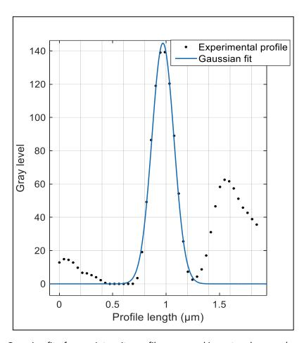
Figure S1. Gaussian fit of mean intensity profile measured in rectangle areas (see Figure 3).
