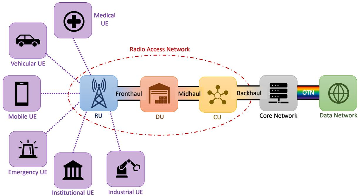
**Figure 1.** Current State-of-the-Art Network Architecture highlighting UE types; the OpenRAN architecture; the identification of the front-, mid-, and backhaul networks; the core and data networks; as well as a depiction of the connectivity between all network elements and regions.
