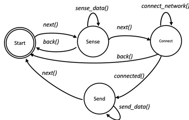
**Figure 3.** The process state machine of healthcare monitoring devices.
