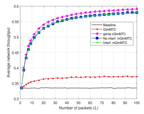
**Figure 7.** Average network throughput  $\times L$ , for K = 600, and M = 100.
