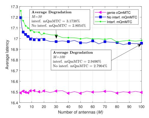
**Figure 4.** Average latency  $\times$  *M*, for *L* = 10 packets, and *K* = 400.
