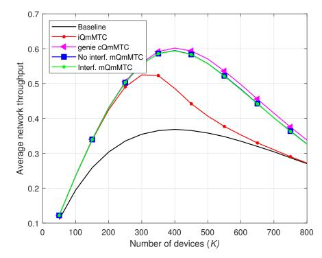
**Figure 3.** Average network throughput  $\times K$ , for L = 10 packets, and M = 100.
