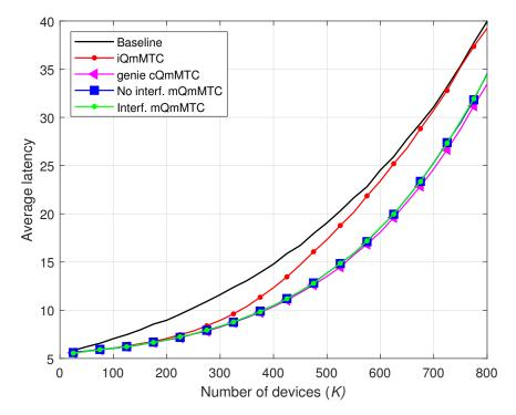
**Figure 8.** Average latency  $\times$  *K*, for  $L_k \sim U(1,10)$ , and M = 100.
