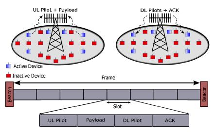
**Figure 1.** Illustrative representation of the adopted cellular mMTC network with IoT devices employing GF RA protocol for their activation and payload data transmission.
