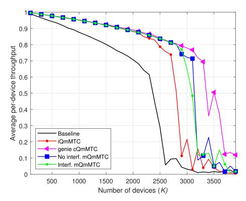
**Figure 10.** Average per-device throughput  $\times K$ , for  $L_k \sim U(1,10)$ , and M = 100.
