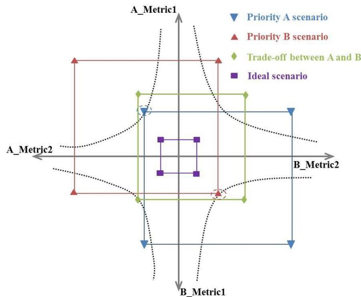
In this 4D coordinate, the dotted lines are plotted in quadrant one and four are the Pareto fronts. The rectangles are signs of metrics balance for different scenario requirements according to the decision maker. In this 4D Pareto front,  $A\_Metric2$  and  $B\_Metric1$  axes are reversed to make the plot clearer, and quadrant two and three are used as the auxiliary quadrant to help locate the rectangle tradeoff markers.
