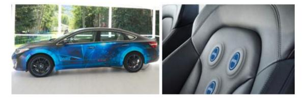
**Figure 4.** Toyota's DARV 1.5 and Plessey's EPIC Seat Sensors. Image credit: Toyota's Collaborative Safety Research Center [42] and the Motor Report [43].
