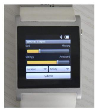
Figure 1. Smartwatch manual data collection interface.
