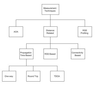
Figure 1. Classification of measurement techniques for localization algorithm.
