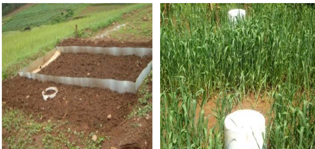
Figure 2. Static gas sampling chamber collar installed in the field adjacent to runoff plots (left) and static chambers with covers on the top ready for gas sampling (right).
